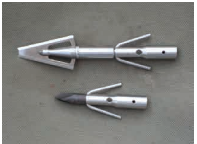
The original Muzzy Gator Getter Arrow (bottom) and Pieter's modification which now carries a standard Broadhead which has had the pointed tip ground to a chisel shape giving better penetration. Note the extension tube which attaches the modified broadhead.
