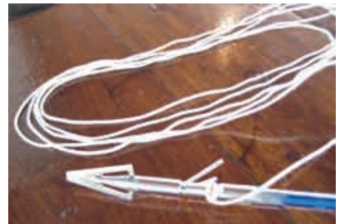
The broadhead/fishing arrow combo with the tether line attached. Tying the cord to the arrow head with a low profile knot is essential so as to reduce any unwanted drag when the arrow enters the skin. Note the wire barb. This and the 600lb Gator Cord will hold just about anything.
